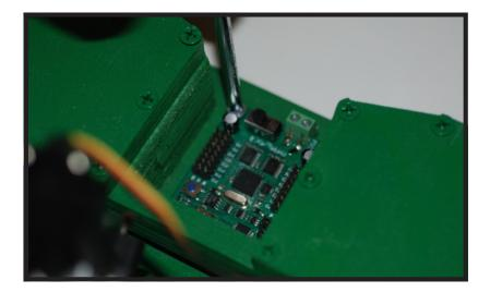
**Step 22**Tighten down the screws to fasten the parallax board to the wooden base. Take care not to overtighten the screws.
