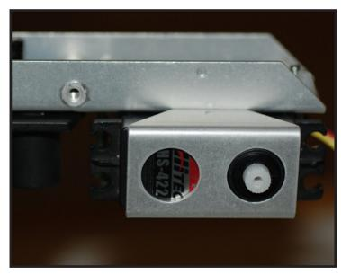
Step 10 Place the 2-hole metal link over the servo you just attached.
