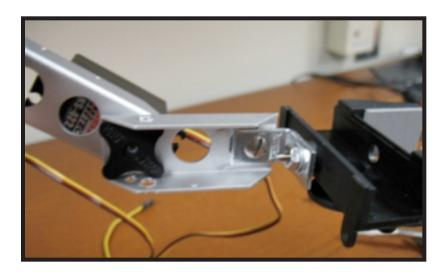
Step 20 Now attach the gripper assembly to the rest of the arm as shown, using the nylon washer and servo connector.
