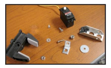
Step 16 Now gather together the gripper hand, another servo motor, the angle link, the #8 and #6 screws, nut and washer, and the 3-hole arm link with its connector and white nylon washer (not pictured).
